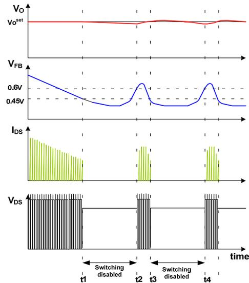
Figure 22. Burst-Mode Operation
