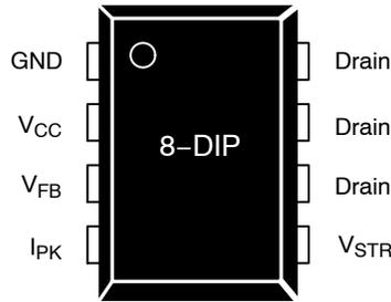
Figure 3. Pin Configuration
